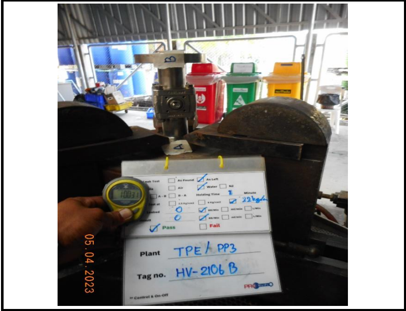
Seat leak test (As Left)
