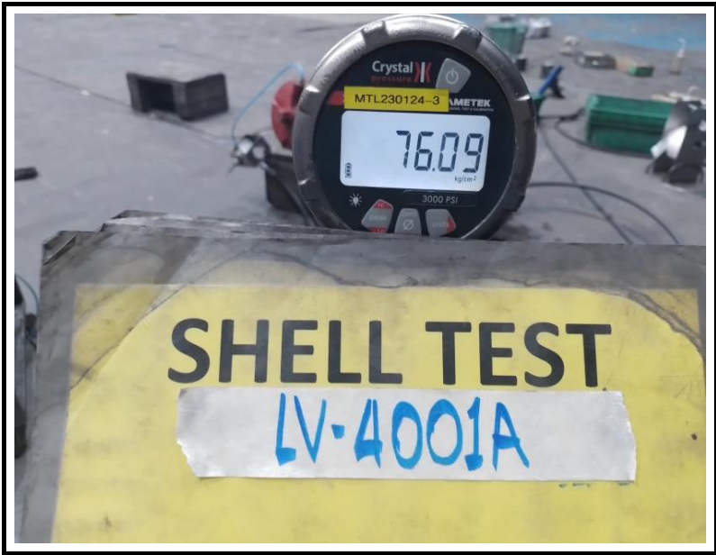
Shell Test (As Left)/No visivle leakage
