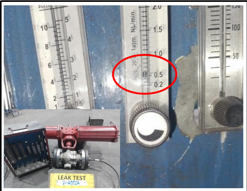
Seat leak test (As Left)/Valve leak 500 CC/min
