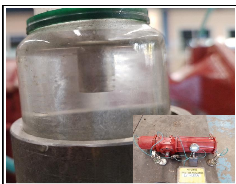
Leak test actuator (As Found)/No visible leakage
