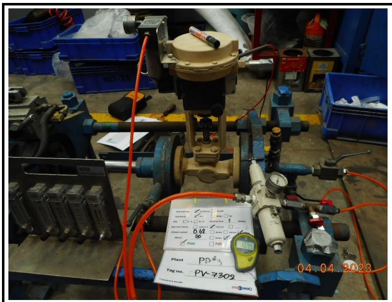
Seat leak test (As Found)
