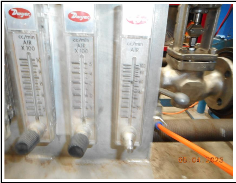
Seat leak test (As Left)
