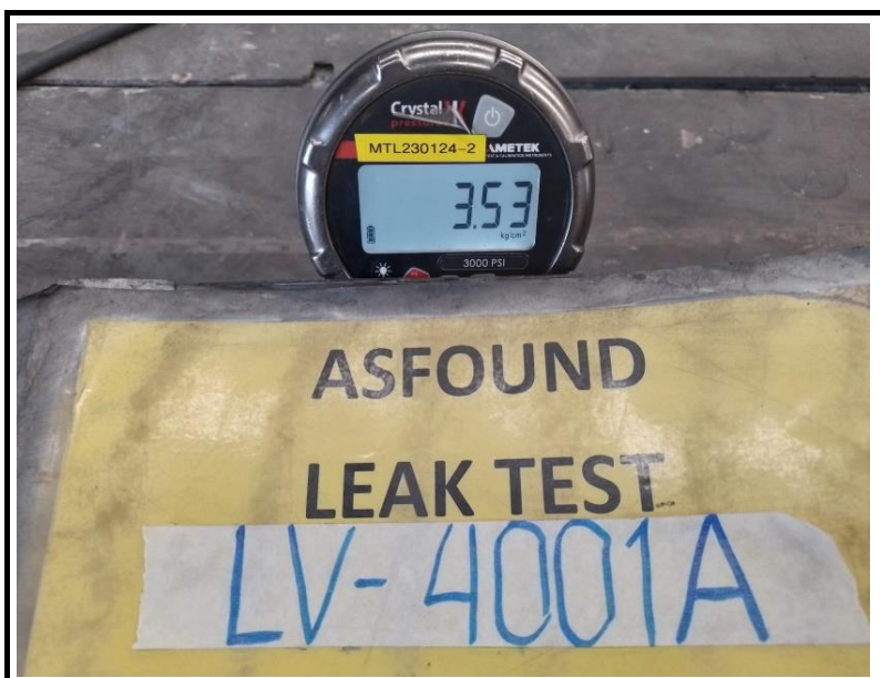
Seat leak test (As Found)/Valve leak 4.2 liter/min
