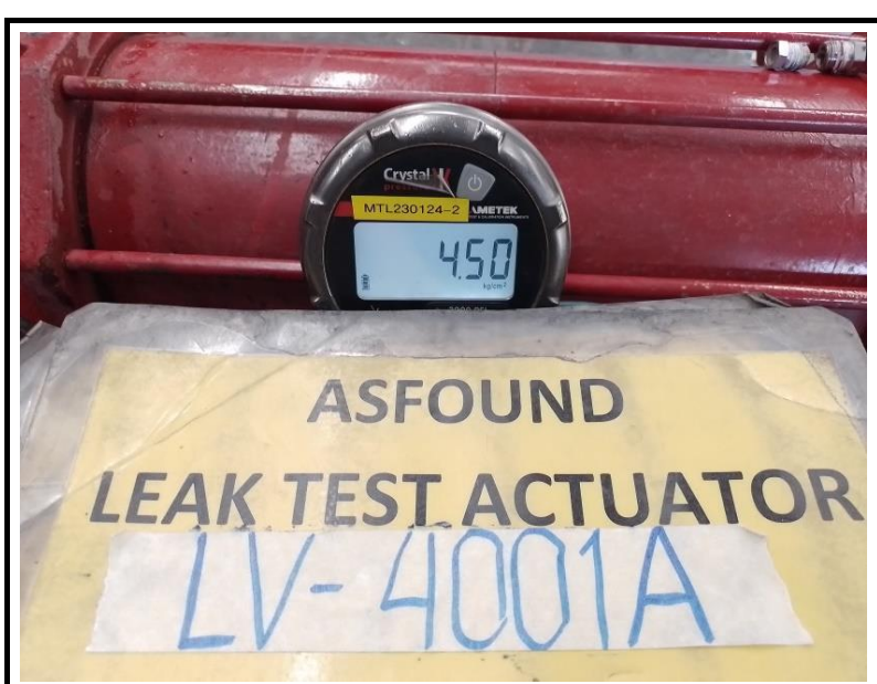
Leak test actuator (As Found)/No visible leakage
